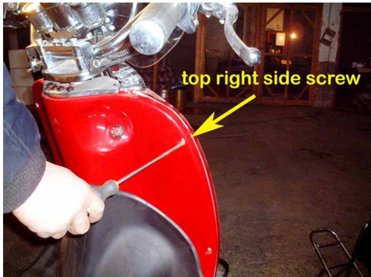
And 3 more on the right back side and they all have to be removed. The picture above shows removing the upper one. A Phillips screwdriver is needed for all these.
