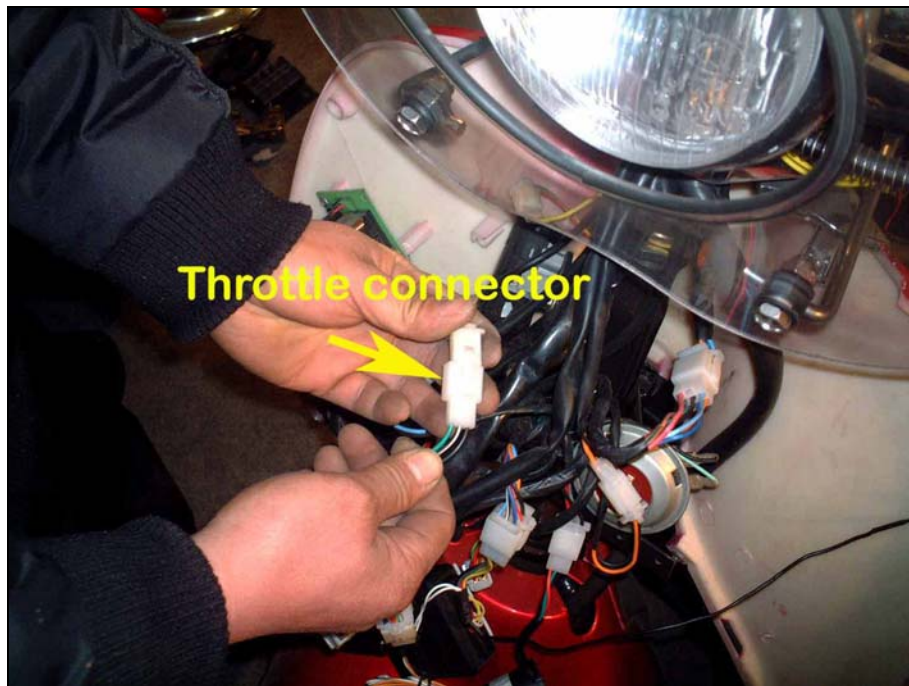
The above photo shows the throttle 3 pin connector. Note the colors (green-black and white-black). This connector must be unplugged before removing the throttle.
