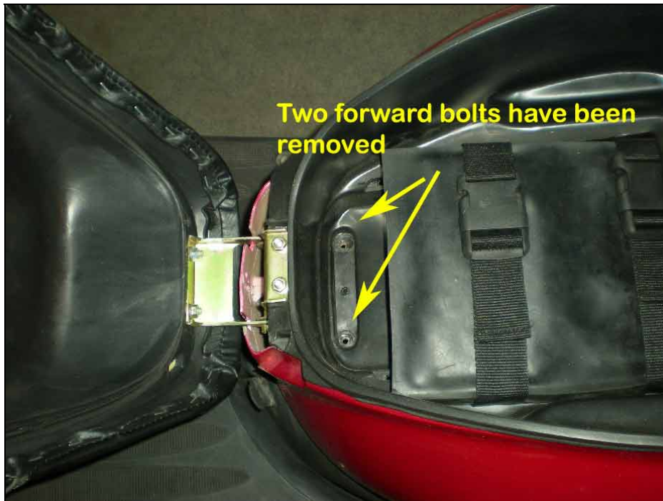
The two pictures above show that the nuts and bolts have been removed
